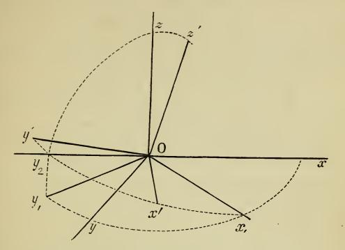
plane of x'y', it also is perpendicular to  $Ox_1$ . Hence  $Ox_1$  is perpendicular to the lines Oz and Oz', and is therefore perpendicular to the plane in which they lie, and therefore perpendicular to  $Oy_1$ ,  $Oy_2$ . Hence by Euclid, XI. Def. 6, the angle  $y_1Oy_2$  is the angle between the planes of xy and x'y'. Let this angle be called  $\theta$ , and let the angle between Oxand  $Ox_1$  be called  $\phi$ , and the angle between  $Ox_1$  and Ox' be called  $\psi$ .
